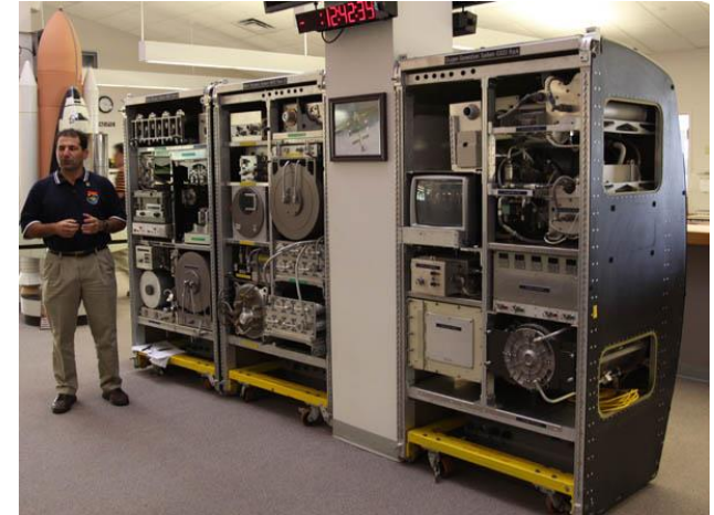
ISS Water Recovery System
