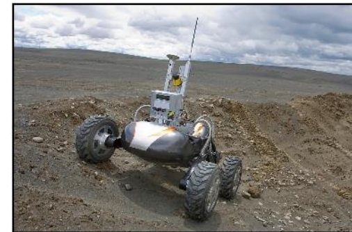
Scarab rover designed to prospect for ice in lunar craters (CMU)
