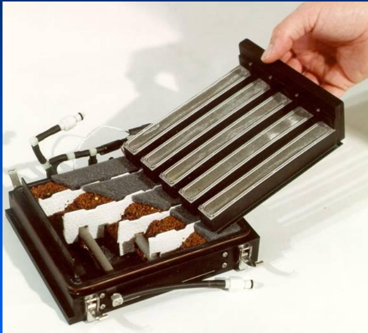
Porous steel tubes surrounded by arcillite rooting media with time-release fertilizer
