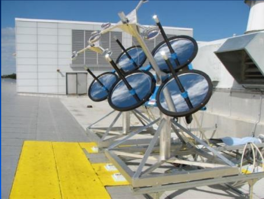
2 m 2 of collectors on solar tracking drive -- roof of Space Life Sciences Lab, KSC
