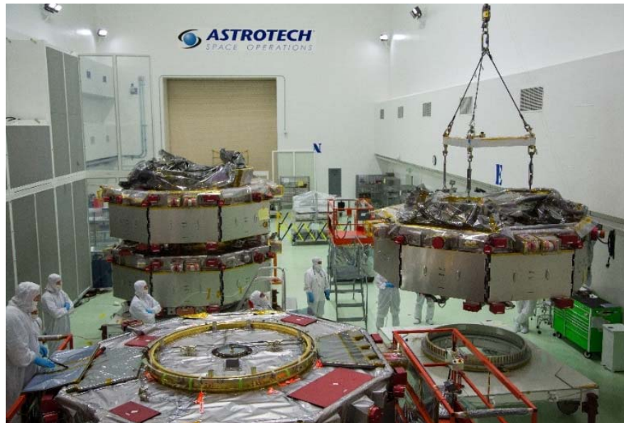
MMS Team performing stacking and final check-outs at AstroTech Payload Processing Facility
