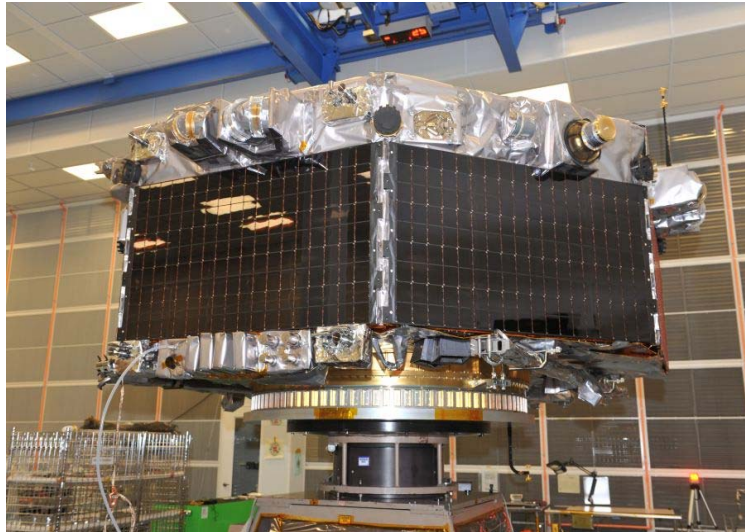
Observatory #1 - Mass Properties Test & Balancing
