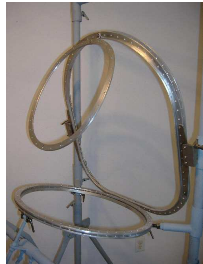
Figure 9. NDX-2 Helmet, Waist, and Rear-Entry rings
