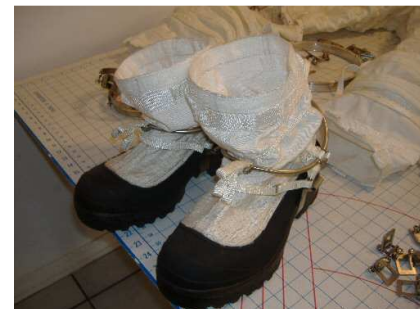
Figure 16. NDX-2 Boot Assembly
