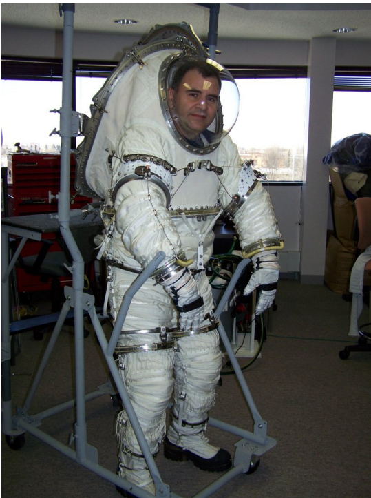
Fig 6. NDX-2 suit during preliminary human-rated testing.
